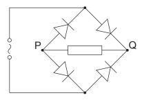
The conventional current in the load resistor
